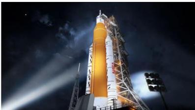
*The Space Launch System (SLS), in its Block 1 crew vehicle configuration that will send astronauts to the Moon on the Artemis*
